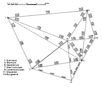
Fig. 2.1.6. The diagonal weight-coefficients of the adjusted directions and of a number of  $\ln v$ 's.
