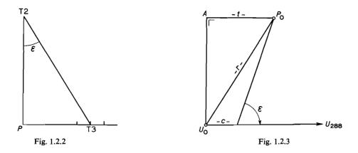
distance between both theodolites is taken equal to the distance between the Jäderin mark and the underground mark (Fig. 1.2.2). With the Wild T2 the angle between the reading index on the Jäderin mark and the sighting index on the telescope of the Wild T3 is measured in two diametrical positions of the alidade of the Wild T3. The mean angle  $\varepsilon$  is the correction which should be applied to the angle measured with the Wild T3.
