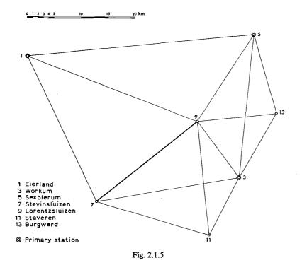
The objective of the base extension network is the determination of a number of distances  $\underline{s}_{i,j}$ . The measurement of the base gives as result the distance  $\underline{s}_{7,9}$ . The measurement of the extension network results in a number of derived quantities  $\underline{v}_{7,9;i,j}$ , defined as follows:
