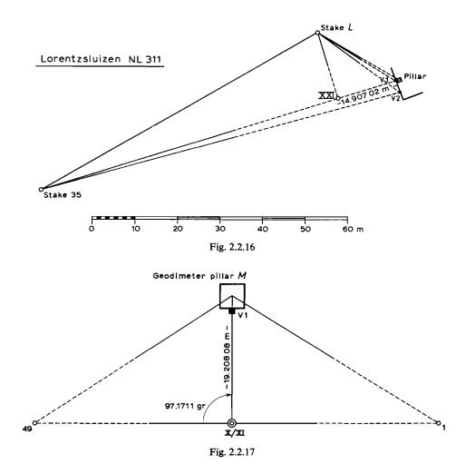
was set up on the geodimeter pillar and on the junction pillar. At both points the three directions as indicated in Fig. 2.2.17 were determined. The distance geodimeter pillar – junction pillar was calculated from the two triangles and the mean of the two values thus obtained was taken.
