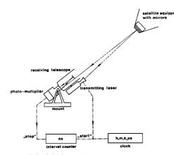
Principle laser distance measurement
