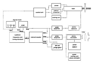
Diagram laser distance measurement equipment
