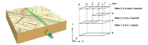
Figure 13 Illustration of 3D (a) railway tunnel crosses several land parcels and (b) temporal concept – changes of state of a subdivision – in a cadastral register (Döner et al, 2011).
