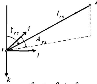
$l_{rs}$  is the length of side  $r, s$ ,  $A_{rs}$  is the angle, measured clockwise, from the  $i$ -axis in the  $i, j$ -plane and  $\xi_{rs}$  is the angle measured from the negative  $k$ -axis (see [ 40 ] ). These quantities do not belong to the set of estimable quantities mentioned before, nor can they be computed from variates introduced earlier. Therefore they belong to the S-base. Thus computations make use of :
