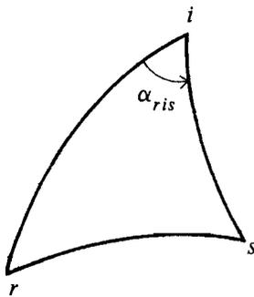
simplified interpretation by the assumption that the k-axis always points towards the centre of the sphere. Measurement in point  $i$  gives the angle between large circles connecting  $i$  respectively with  $r$  and  $s$ .
