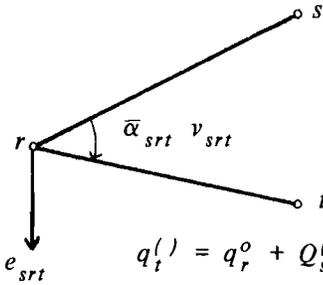
$e_{srt}$  is the unit vector normal to plane  $s, r, t$  and thus perpendicular to side  $r, s$ , so, only one directional component is undetermined. This component is not estimable and also not expressible as a function of variates introduced as yet. So it belongs to the S-base, therefore, we use  $e_{srt}^o$ . Then point  $t$  is :
