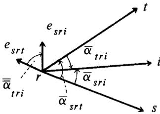
Points  $r, s, t, i$  are not all in one plane. According to section 3.3.1 the measurable quantities are the angles  $\bar{\alpha}_{srt}$ ,  $\bar{\alpha}_{sri}$  and  $\bar{\alpha}_{tri}$  and the ratios of lengths  $\ln v_{srt}$ ,  $\ln v_{sri}$  and  $\ln v_{tri}$ .
