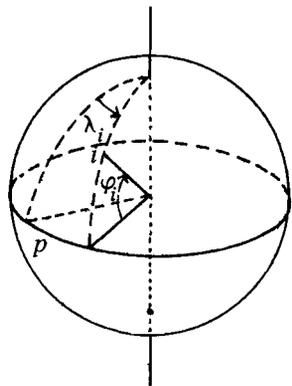
The angle between  $R_p$  and the orthogonal projection of  $R_i$  on the equatorial plane will be denoted by  $\lambda_i$ , the second coordinate of  $i$ .  $\varphi$  and  $\lambda$  are counted as indicated in the figure. The coordinate computation will start from point  $r$ . The coordinates of this point do not belong to the set of estimable quantities nor can they be computed
