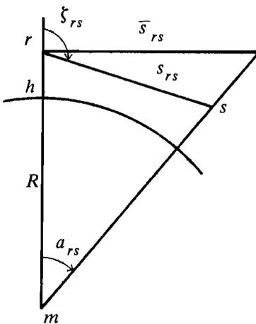
Suppose an instrument has been set up at station  $r$  and the distance is observed to  $s$ , with zenith angle  $\xi_{rs}$  which is supposed to be corrected for refraction.
