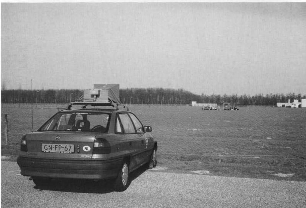
Signal generator. Jamming test at NLR (11 March).
