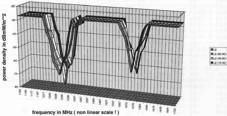
Power was increased 2 dB each time for frequencies between 1118 and 1685 MHz unless stated otherwise. All other steps were 10 dB. The power loss is about 40 to 50 dB per-to-signal ratio.
