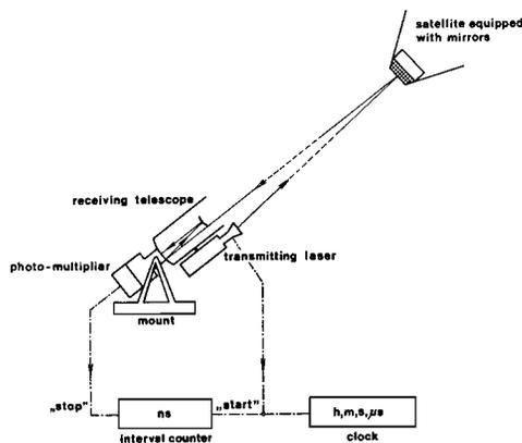
Principle laser distance measurement
