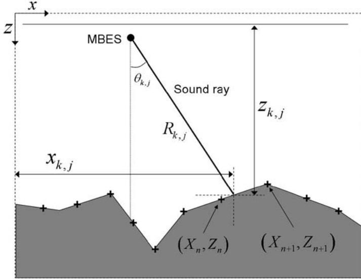
Figure 3. Illustration of the model for  $t_{k,j}$ . On the right side of the MBES we show the path of a sound ray through water column. The ray impinges at the seafloor in between the grid points  $X_n$  and  $X_{n+1}$  at coordinates  $(x_{k,j}, z_{k,j})$ .  $t_{k,j}$  is calculated as  $2R_{k,j}/c$ .
