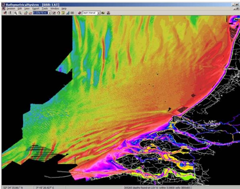
*Figure 1. Screen dump of Bathymetric Archive System (BASRBB) on Level of Visualisation (LOV) 6 showing the Southern North Sea, coloured by depth. The area is characterized by sand waves and mega ripples. To better understand the dynamic behaviour of these sand waves studies are underway by various groups at Dutch universities and government institutions.*
