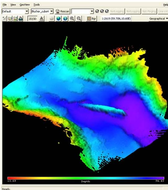
Figure 13. A terrain model made from depth points.
