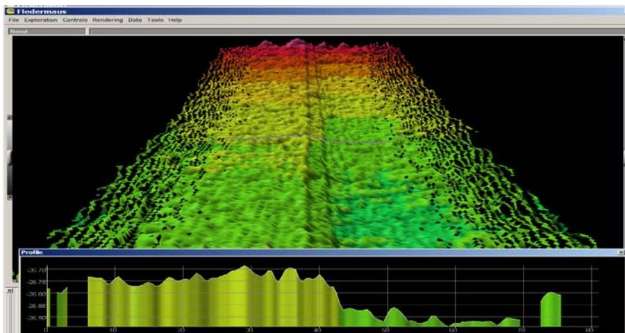
Figure 6. Example of dual-head transducer misalignment error artefact.
