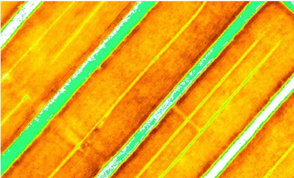
*Figure 12. With a suitable legenda, the 50 cm AHN-2 grid shows ditches, drains and other topography of interest to water management with a high level of detail (Hoogheemraadschap De Stichtse Rijnlanden (HDSR)).*
