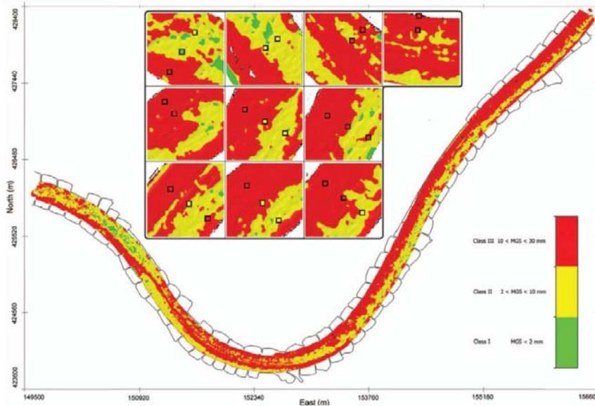
Figure 8. Acoustic classification map for an area of the Waal, close to St. Andries. The three colors indicate the three acoustic classes. The results of the sample analysis are shown by the squares. MGS indicates the mean grain sizes.
