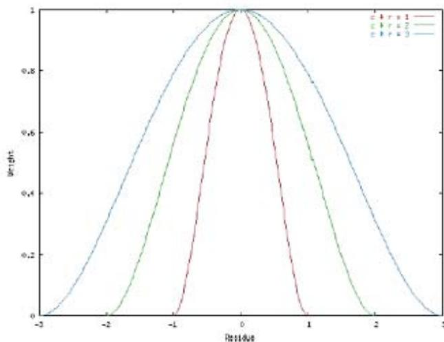
Figure 11. Tukey weight functions of residue and weight.
