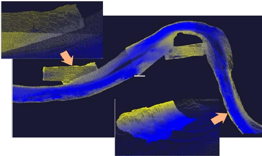
*Figure 6: Point Cloud of a Bathymetry dataset. The inset top-left indicates aliasing errors caused by the regularity in data and the sampling algorithm, the other inset shows a region where point sampling density is much larger than its surrounding area.*
