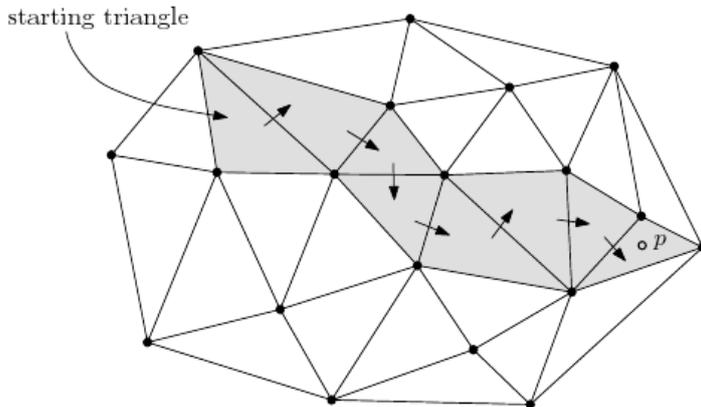
Figure 5. The WALK algorithm for a triangulation.
