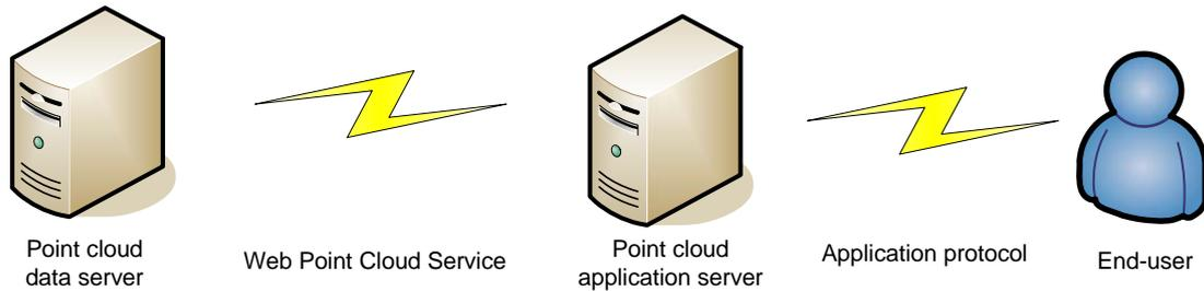
Figure 5. Point cloud distribution structure.
