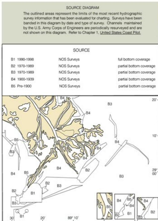
Figure 4. Example source diagram (courtesy NOAA).
