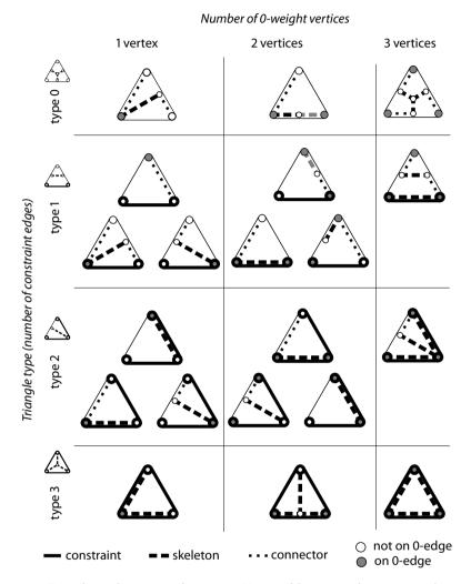
Figure 4.23: Triangles with zero-weight vertices. Unmovable vertices, having a weight = o, are coloured gray. Skeleton segments that will be created are in black, skeleton segments that will not be created are visualised with gray (*e. g.* triangle type-0-2-vertices).
