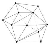
(d) The constrained triangulation of the set of points and segments. The dashed lines are the edges of the triangulation of *S* that are removed since they are not conform to the input segments.
