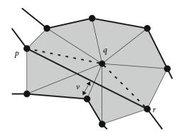
Figure 2.10: Line simplification using a constrained triangulation. The original part of the line, formed by the vertices p, q and r is simplified into  $\overline{pr}$ , if the separation distance v between the new line and the other lines is large enough. The triangulation is used to be able to define and check this distance v. Taken from Dyken et al. (2009).
