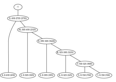
Figure 4.4: The tGAP face-tree, corresponding to the data set of Figure 2.18a, encoding how area features are progressively merged.
