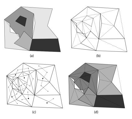
Figure 3.12: (a) Six polygons form the input planar partition. (b) The constrained triangulation of the boundaries of the input polygons. (c) The dual graph of the triangles is drawn with dashed lines; the dark points are the points from which the walk in each polygon starts. (d) The result contains triangles that are not flagged (white triangles). The white triangle on the right is not a problem since it is a 'universe' triangle.
