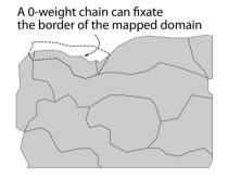
Figure 4.22: Fixating the border of the domain can be performed with 0-weights. Note that there should at least be 1 non-zero weight neighbour, otherwise no split can take place.
