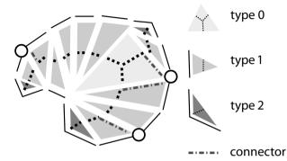
(b) Connectors and skeleton edges are created locally, *i. e.* generated for each triangle individually. Which connectors and skeleton edges are generated is dependent on the type of triangle. To prevent duplicate connectors for neighbouring triangles, the connectors are only generated going outward of a node (where an external chain is incident) when going counterclockwise around a triangle.
