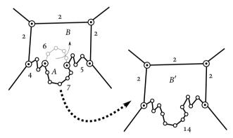
(b) Unwanted nodes also result from merging two polygonal areas. Furthermore, the average number of coordinates per boundary increases.
