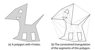
Figure 3.9: A polygon and a possible triangulation. Observe that polygons in GIS can contain holes (many for certain applications) and that one hole touches the outer boundary of the polygon.
