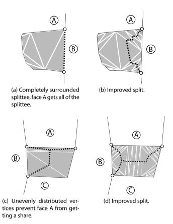
Figure 4.27: (a) & (b): Face A completely surrounds the splittee and gobbles it up. (c) & (d): On the boundary of the splittee, the vertices are distributed unevenly, leading to small triangles in front of face A: these triangles prevent face A from getting its fair share of the splittee.
