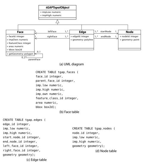
Figure 2.17: An UML diagram and corresponding table definitions in SQL for the classic tGAP structure.
