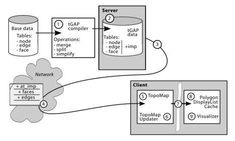
Figure 5.8: Visualisation pipeline for progressive data streaming.
