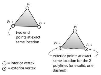
Figure 4.10: If taking a short cut leads to a polygonal area that has no area, we put the end points as blockers for  $p_i$ . The result is that  $p_i$  is not removed, as the endpoints of the polylines will never be removed.
