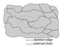
(c) Inside the splittee skeleton edges will be created. The new boundaries will be formed by these edges and the external chains.
