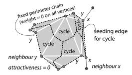
(b) Zero weight edges can lead to cycles in the skeleton graph. The labelling step thus should be modified. In this example x will be propagated onto the edges between two cycles. These edges then will be labelled with x on both sides and removed. The result is that neighbour x gets the complete area of the splittee.
