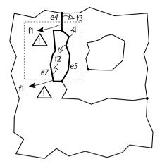
Figure 4.3: Rewriting of face-id's with the use\_tree variant. Edges are retrieved, at imp\_sel = 330, based on their bounding box and the selection rectangle (dashed). After clipping, only the thickest lines are used for forming rings. The most-left ring is formed based on edge 4, 7 and temporary edges stemming from the selection rectangle. Both edges 4 and 7 do not point to the correct neighboring face and rewriting has to take place (face 1 is rewritten using the tGAP face tree as face 8).
