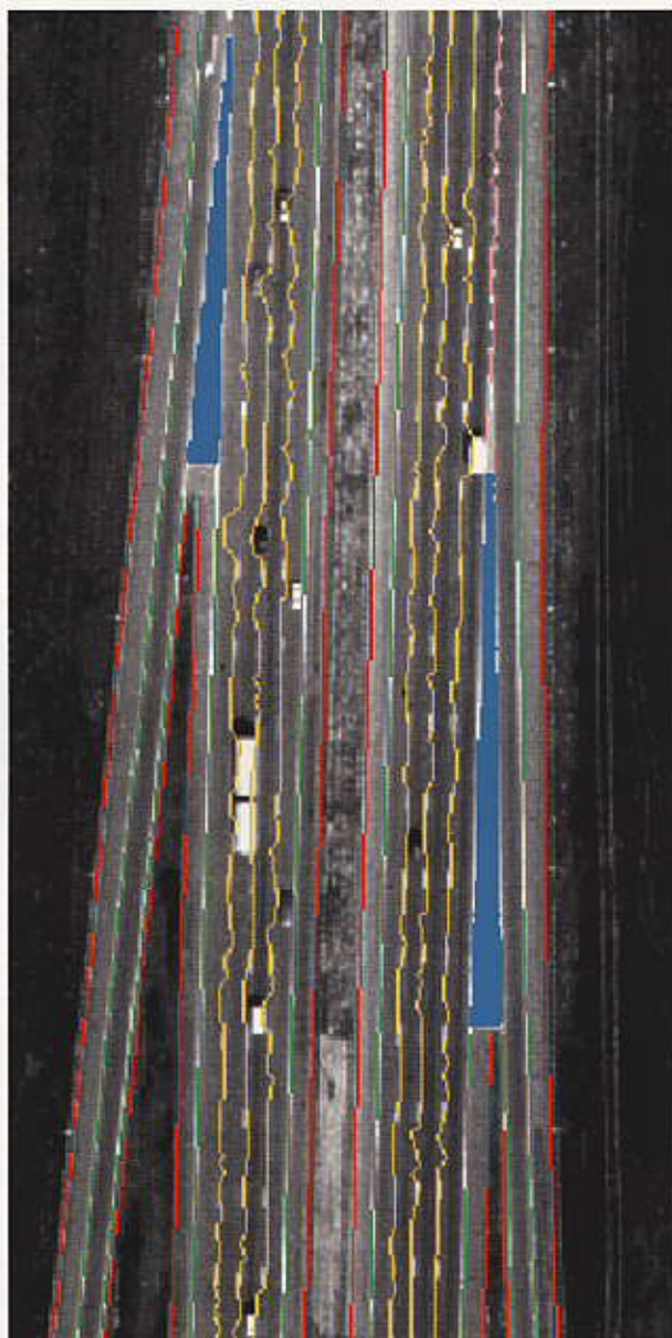
Fig. 4.22 Results at large scale of detection of road sides as components of a Y-junction at medium scale and detection of road markings by contextual reasoning
