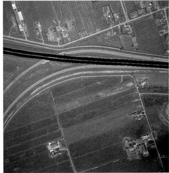
Fig. 5.10 Digital map of the motorway in the outdated situation projected on the aerial image in black
