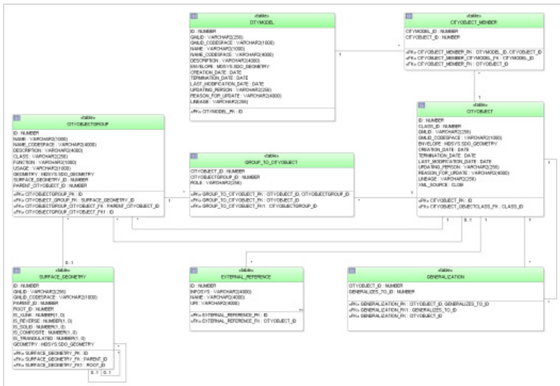
Figure 12. Part of the 3DCityDB schema.
