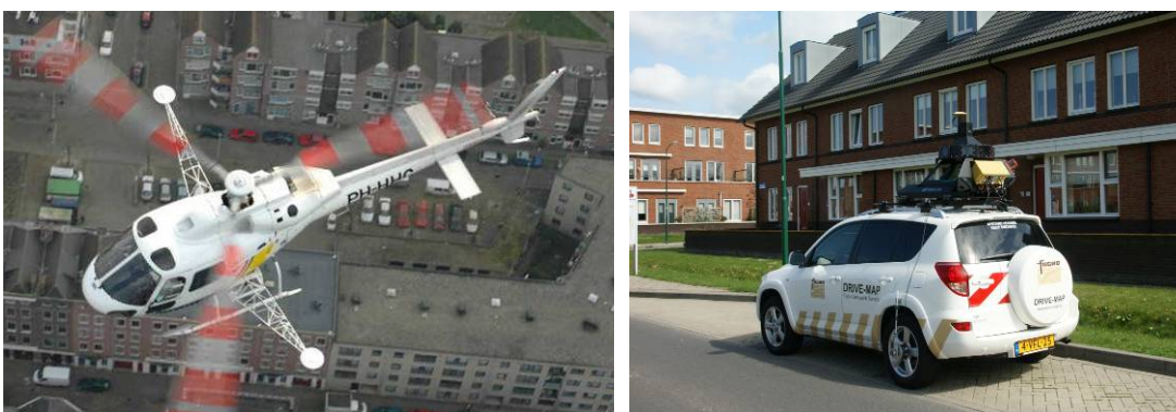
Figure 2. FLI-MAP (helicopter based) and DRIVE-MAP.
