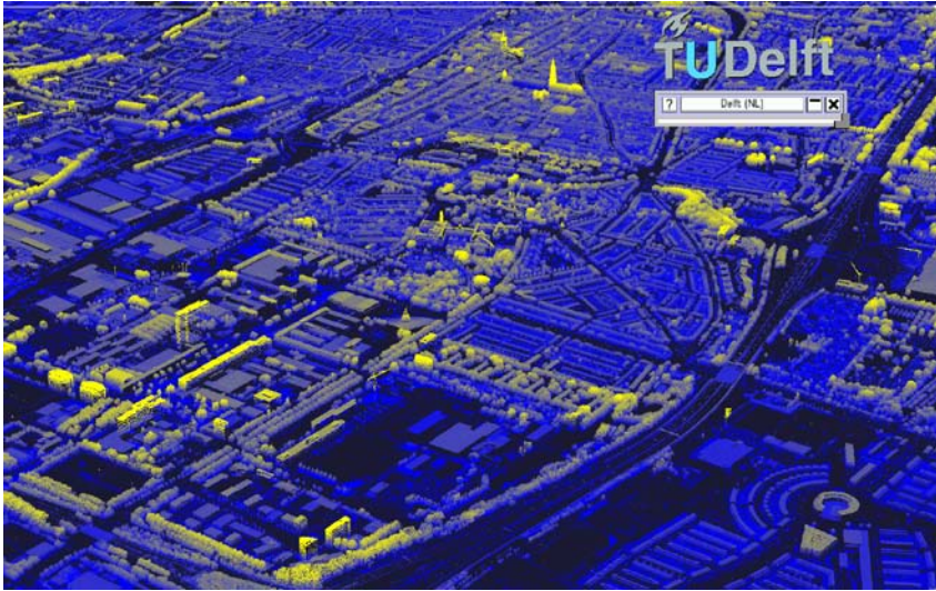
Figure 5: Screenshot of the AHN2 dataset (filtered buildings, no color) surrounding TU Delft campus, ~6 tiles in view at 20 fps @ 1680x1050 (mono), nVidia Geforce 280 GTX. Performance when viewing 100 tiles currently drops to 5 fps.
