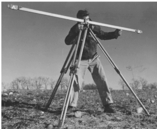
Figure 6: Subtense bar (left) and its principle of distance measurement (right)
