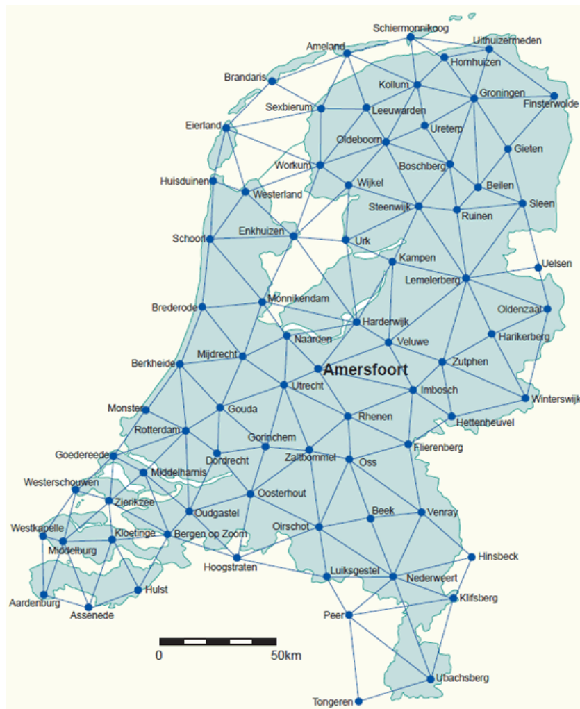
Figure 1: RD-network. The first-order geodetic control network, 1888-1904. See also Figure 13.
