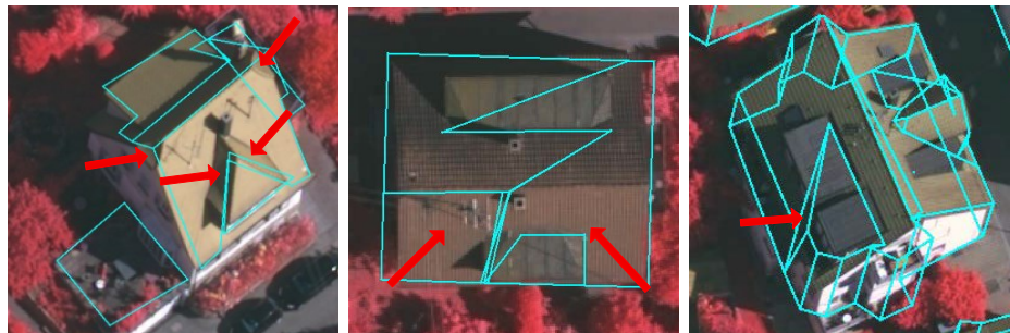
Figure 4-10. Incorrect models reconstructed from erroneous roof topology graph. From left to right: small roofs, wrong segmentations, incorrect combination of planes. (Rottensteiner et al., 2014)
