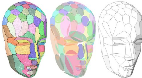
Figure 2-6. Repeatedly cluster faces into local smooth regions and construct approximating polygonal meshes. (Cohen-Steiner et al., 2004)
