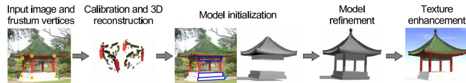
Figure 2-9. Reconstruction of 3D shapes of symmetric piece-wise planar objects via a Markov random field to recover the depth map based on the symmetric line pairs. (Tianfan et al., 2011)
