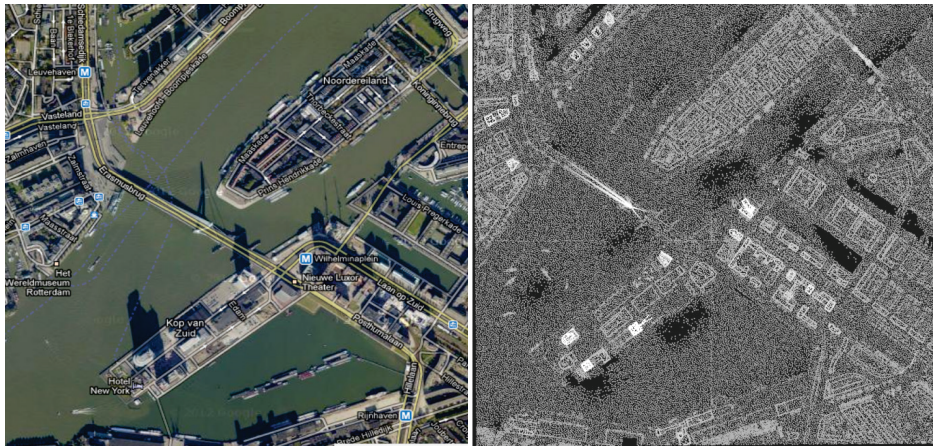
Figure 4.2. Test area (left), image from Google; (Right) ALS data in test area (a black area means no data; the lighter the shade, the higher the point).
