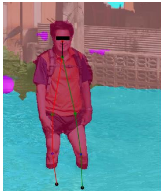
(1) Overlay of semantic segmentation and body keypoints
