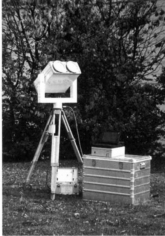
Fig. 1: Transportable Microwave Water Vapor Radiometer (WVR) measuring system of the Institute of Geodesy and Photogrammetry at ETH Zurich in operating position.
