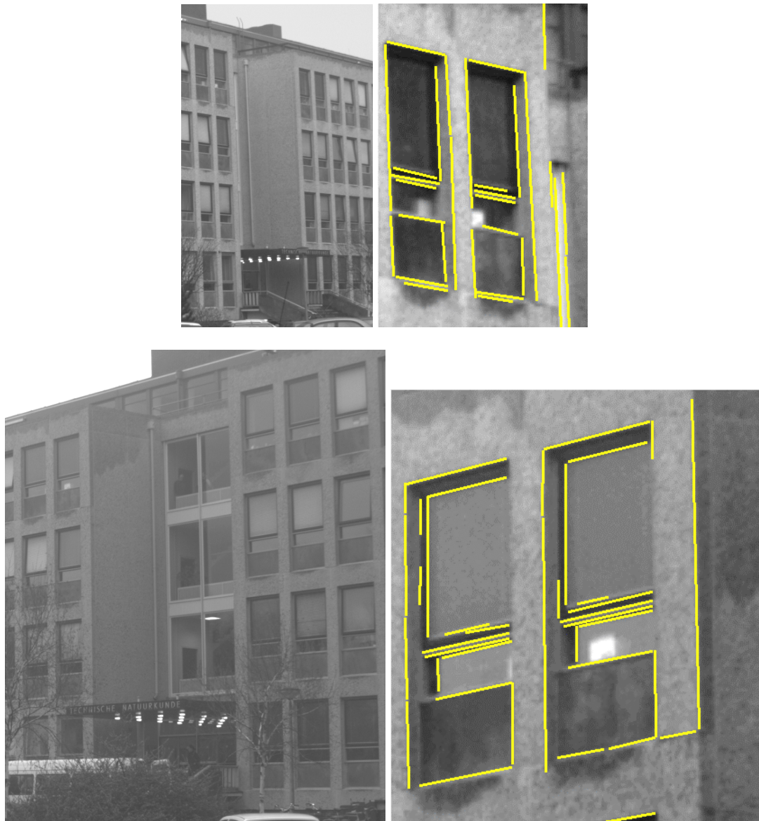
Figure 2: Parts of an image from the left (top) and one from the right (bottom), note the image scale difference. Automatically extracted image lines of the two windows in the upper left corner of the images are shown on the right.
