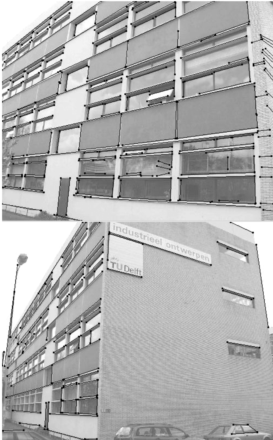
Figure 3: Oblique wide-angle imagery with extracted lines; façade (top) and three-point perspective
