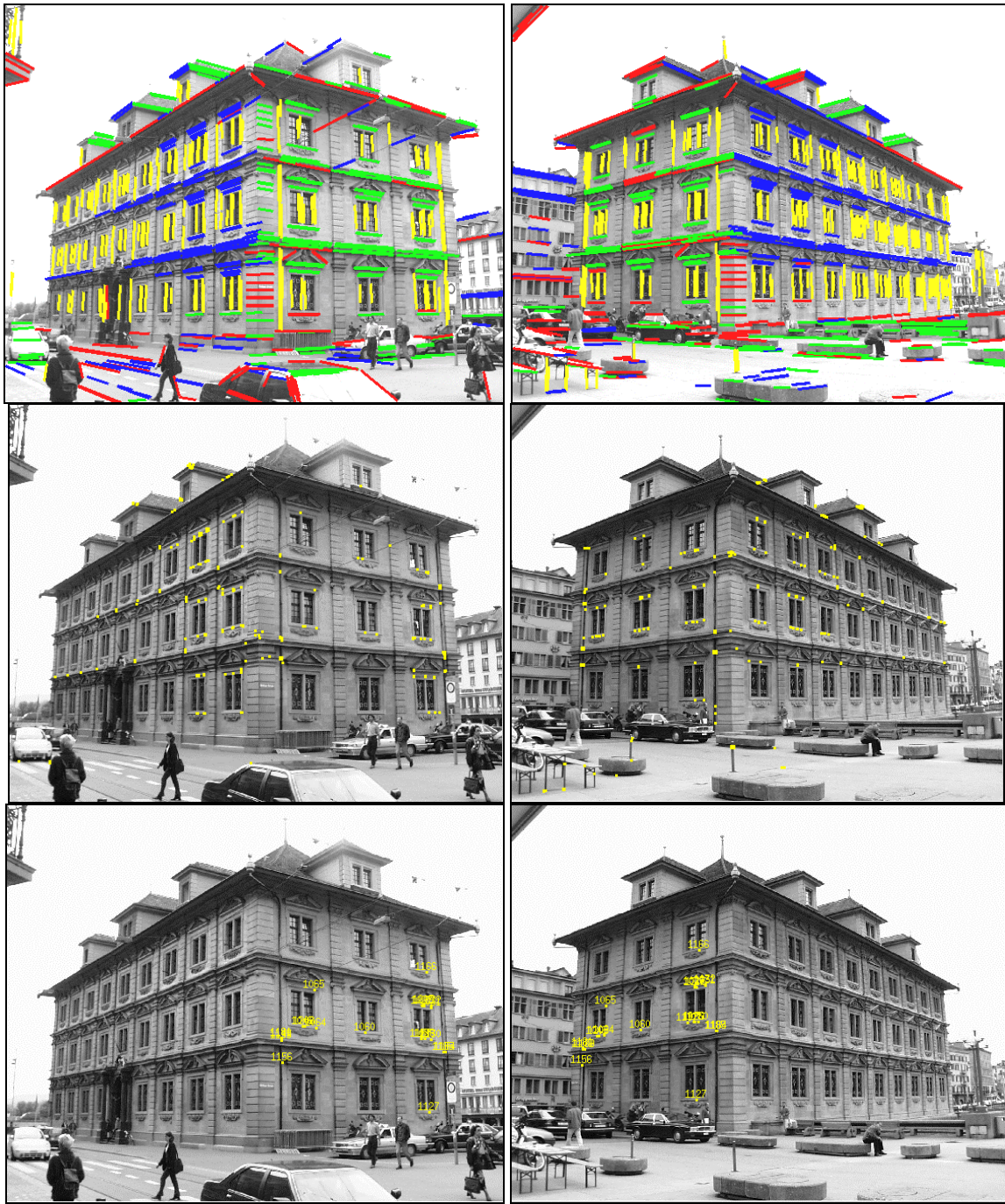
Figure 14: Top: results of line extraction and vanishing point detection of images 6 (left) and 3 (right). Middle: points from line intersections. Bottom: result of correct correspondence detection.
