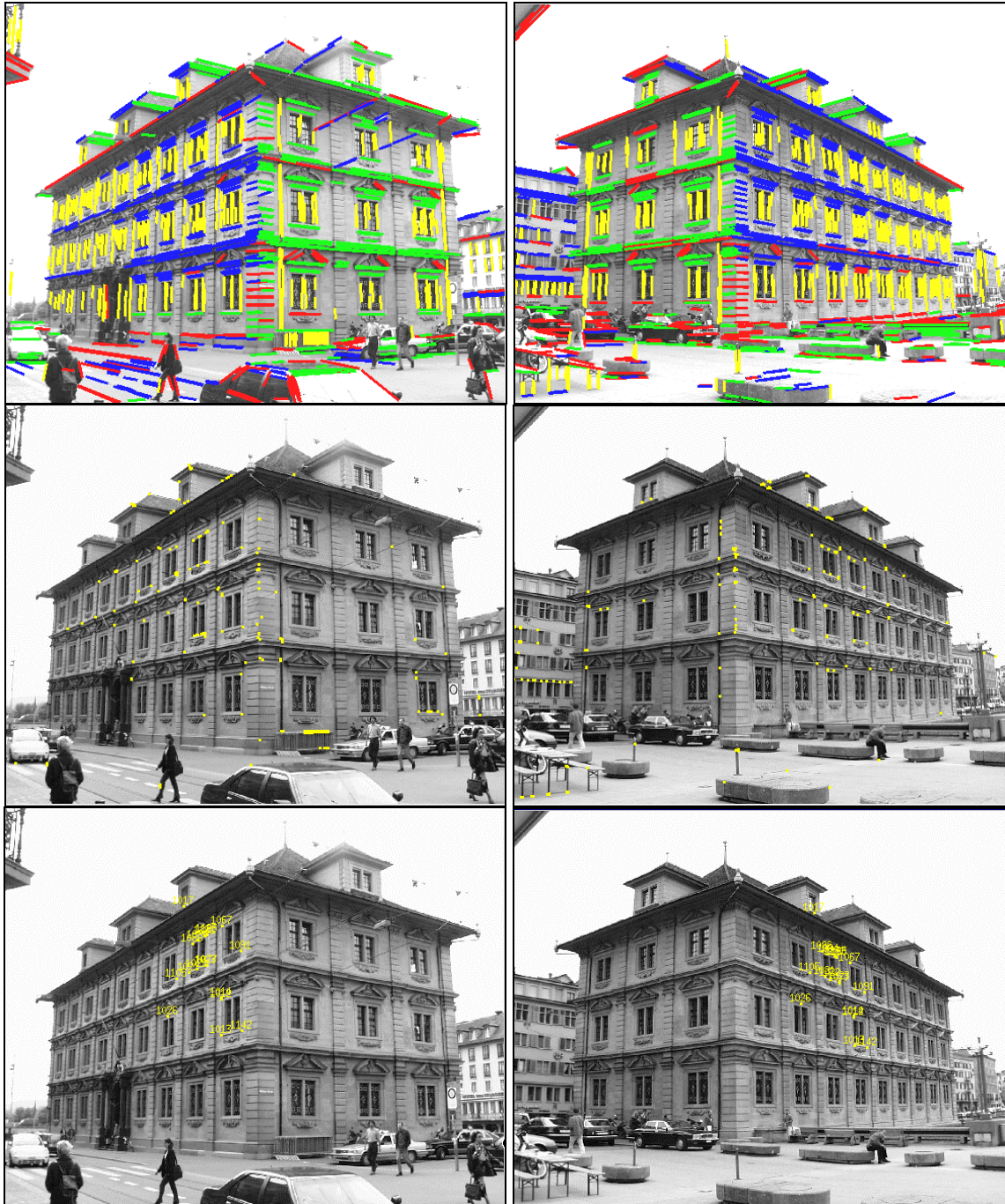
Figure 10: Top: results of line extraction and vanishing point detection of images 6 (left) and 3 (right). Middle: points from line intersections. Bottom: result of erroneous correspondence detection.
