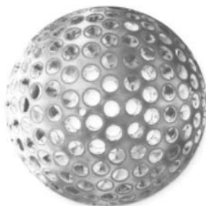
Fig. 2.6: The LAGEOS-I satellite
