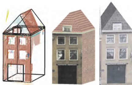
Figure 7.18: Reconstruction of Markt 48 (left: geometry model; middle: textured model; right: by traditional approach)
