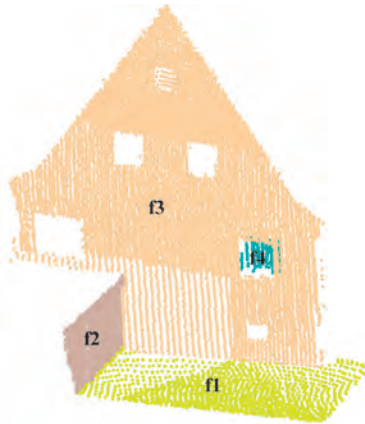
Figure 2.5: A simple building with four features.
