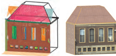
Figure 7.7: Reconstruction of Markt 11 (left: geometry model; right: textured model)
