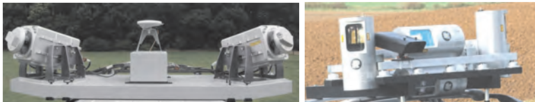
Figure 7.24: The scanner configuration of Lynx (left) and Streetmapper 2 (right) (3DLaserMapping, 2009)
