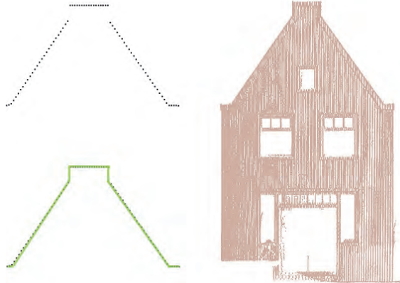
Figure 4.1: Wall outline generation (Left up: upper contour points; left down: least squares fitting; right: generated wall outline).
