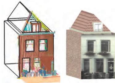
Figure 7.11: Reconstruction of Markt 21-22 (left: geometry model; right: textured model)
