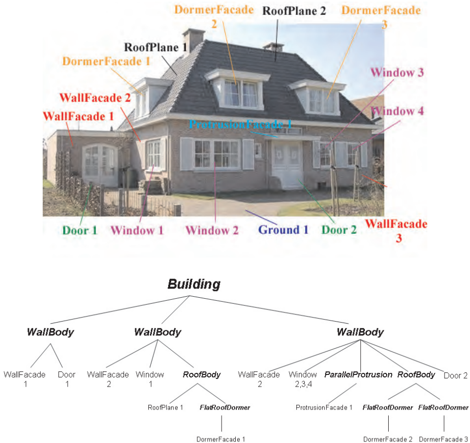
Figure 2.3: Interpretation of a simple house with hierarchical feature composition.
