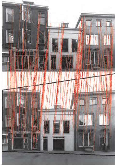
Figure 5.6: Homography estimation using extracted SURF in two images (red lines: linked SURF pairs; black quadrangle: homographic transformed viewing plane of the upper image).
