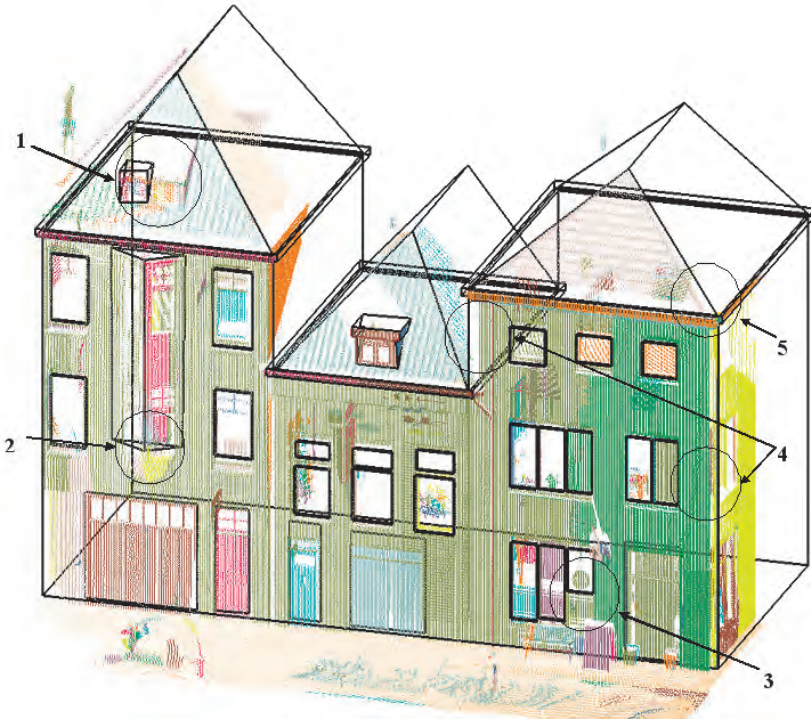
Figure 4.5: Reconstructed polyhedron model of a building facade. Errors occur at: 1. dormer; 2. round corner; 3. window; 4. wall boundary; 5. roof boundary.
