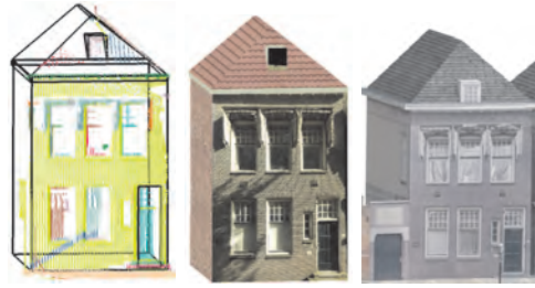
Figure 7.17: Reconstruction of Markt 47 (left: geometry model; middle: textured model; right: by traditional approach)
