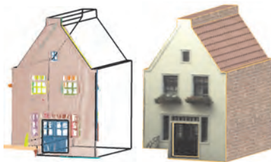
Figure 7.12: Reconstruction of Markt 28 (left: geometry model; right: textured model)
