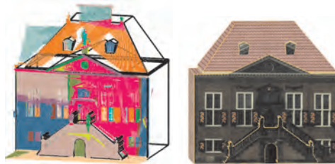
Figure 7.8: Reconstruction of Markt 12 left part (left: geometry model; right: textured model)
