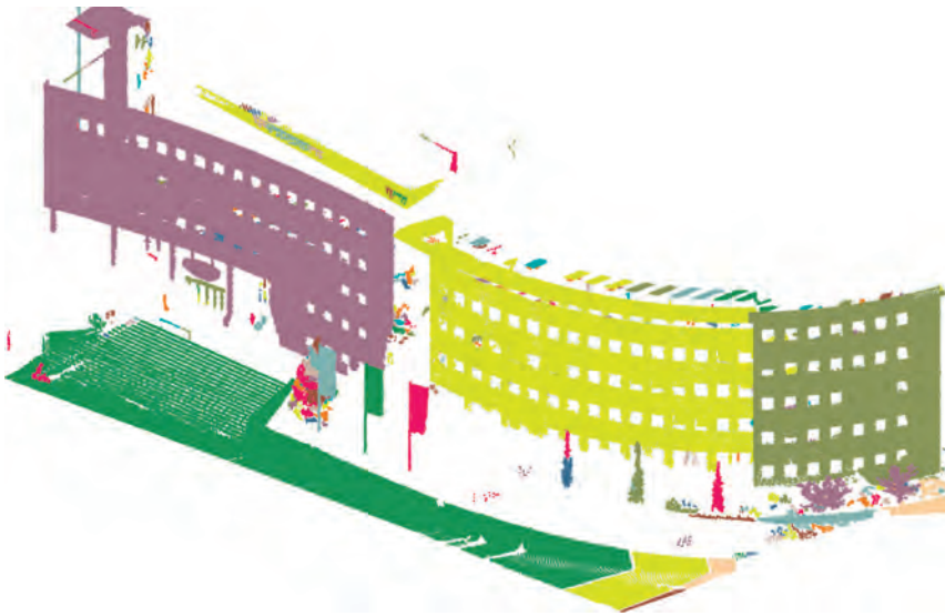
Figure 3.6: Segmentation with the smooth surface method.
