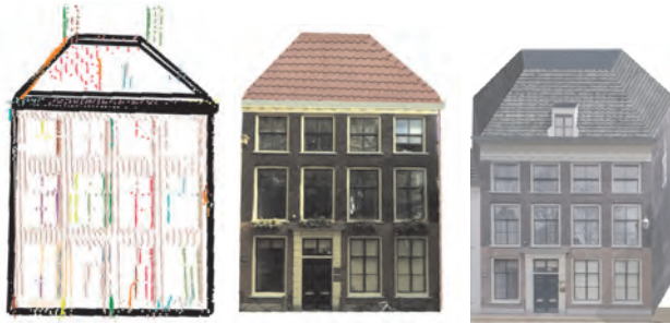
Figure 7.14: Reconstruction of Markt 31-34 (left: geometry model; right: textured model; bottom: by traditional approach)
